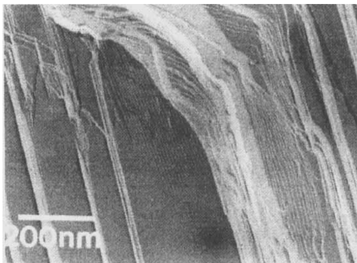
FIGURE 2 Electron micrography of solid phase fracture
